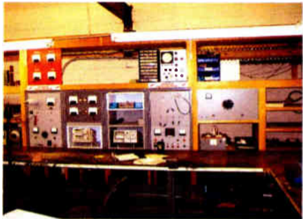
Test bench, with load resistors in the upper right.
