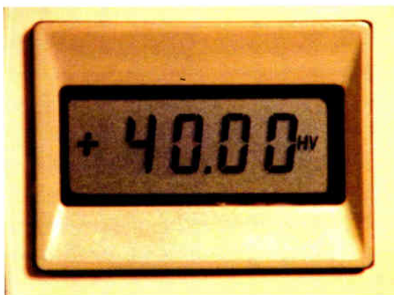
Many DVMS now indicate 40V as "High Voltage."
