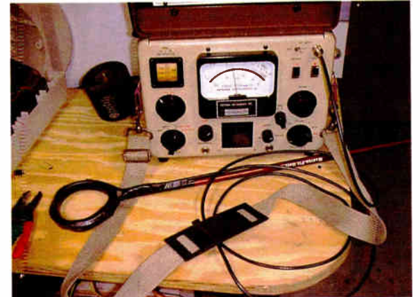
The Ground Loop Sniffer ready for use.
