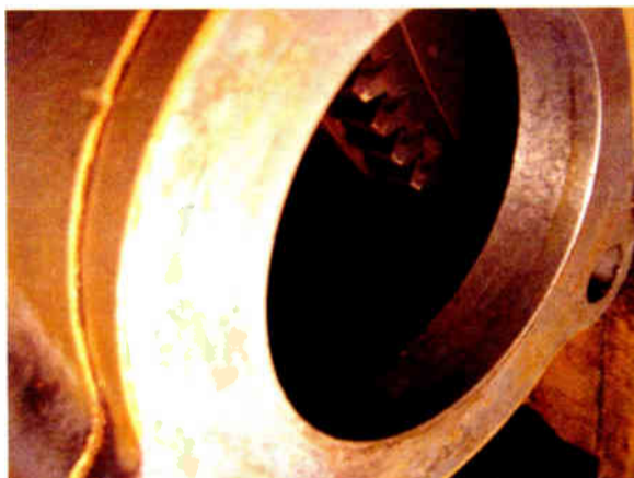
It is important to make sure the flywheel (shown inside the starter ring) is in good condition for a proper mesh with the starter gear.
