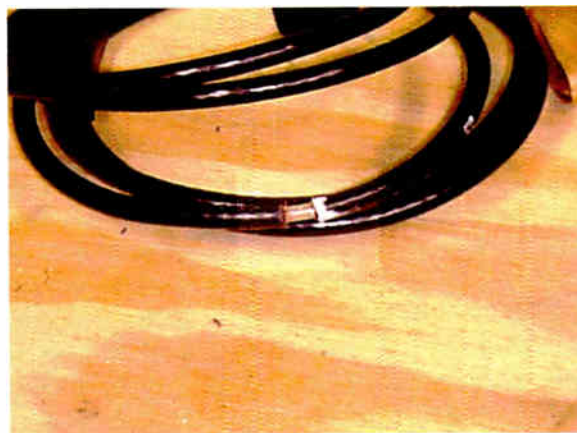
Cutting the shield at the center of the loop.
