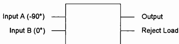
Figure 2: 3dB, 90-degree Hybrid as a Power Combiner
