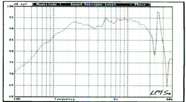
FIGURE 8: 27TAF/G tweeter SPL comparison for two samples.
