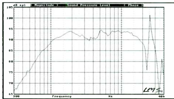
FIGURE 3: 27TAF/G tweeter on-axis frequency-response curve.
