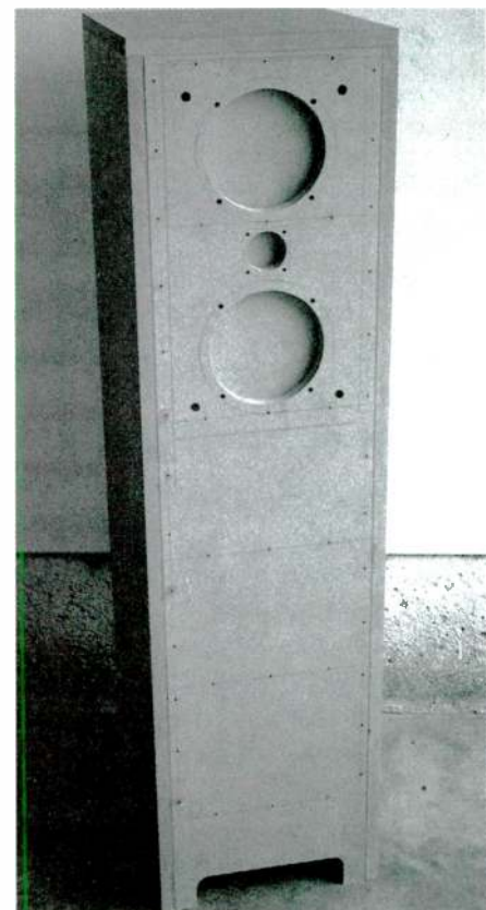
PHOTO 13: Cabinet with front panel installed.
