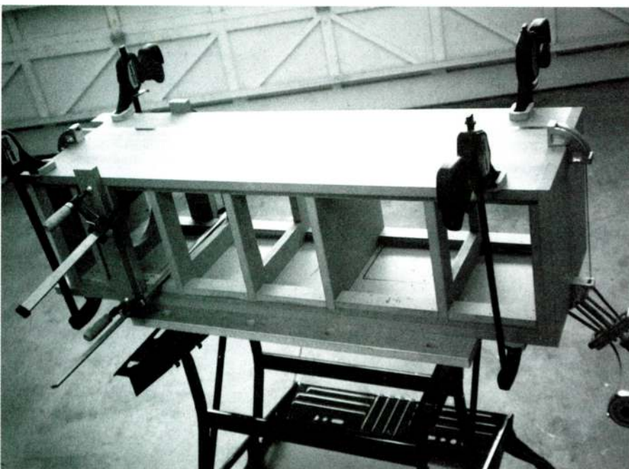
PHOTO 9: Clamped side panels.
