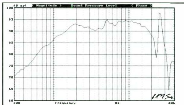
FIGURE 4: 27TAF/G tweeter on-axis frequency-response curve.
