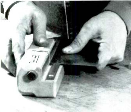
PHOTO 6: Using a special burnishing device to raise the burr.
