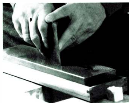
PHOTO 3: Sharpening the edge.
