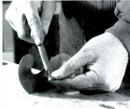
PHOTO 8: Forming the hook on a curved scraper.
