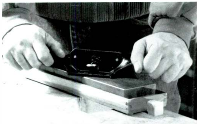
PHOTO 9: Smoothing the base plate on a cabinet scraper using a diamond sharpening stone.
