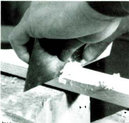
PHOTO 12: Pulling the hand scraper.
