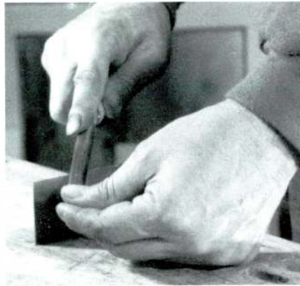
PHOTO 7: Using a burnisher to draw the edge.
