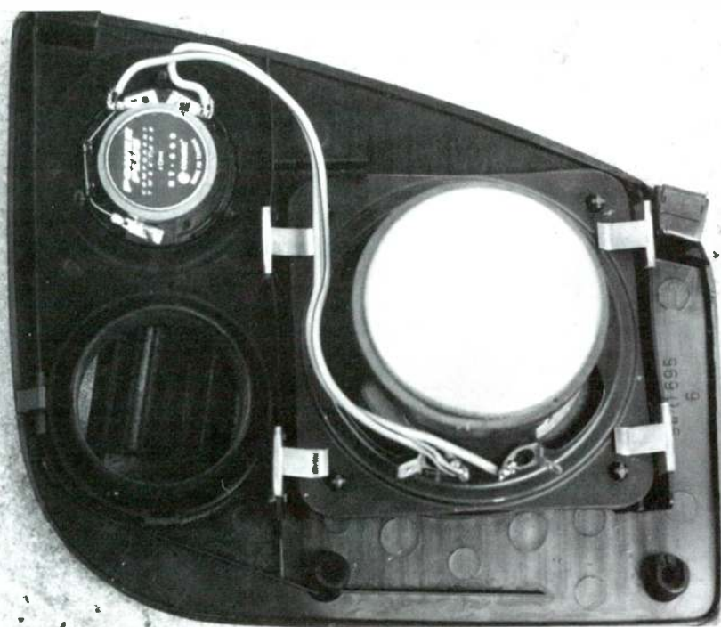
PHOTO 6: Driver's side speaker plate before modification. The original 4" driver used a square mounting plate.
