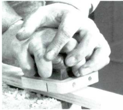
PHOTO 17: A commercial razor scraper, which, like a chisel, does not produce as fine a surface as conventional scrapers.
