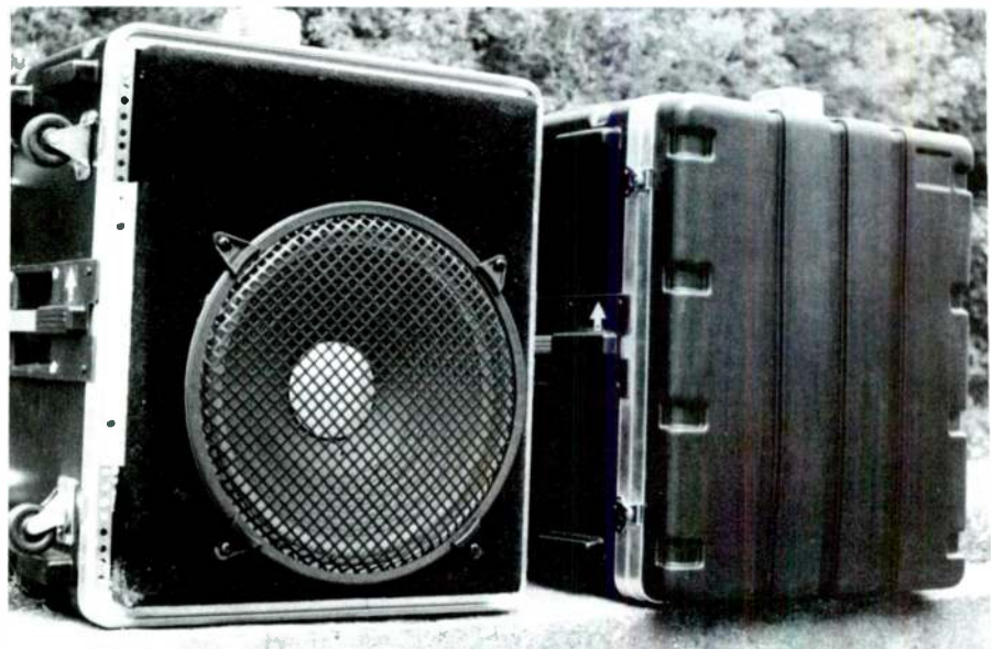
PHOTO 3: Completed bins with and without travel cover in place.
