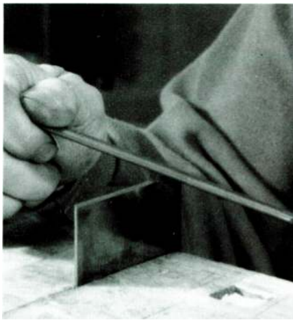
PHOTO 11: Forming a hook on a cabinet scraper blade.
