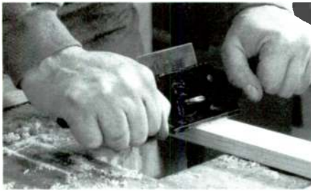
PHOTO 15: Using the cabinet scraper in the pulling mode.
