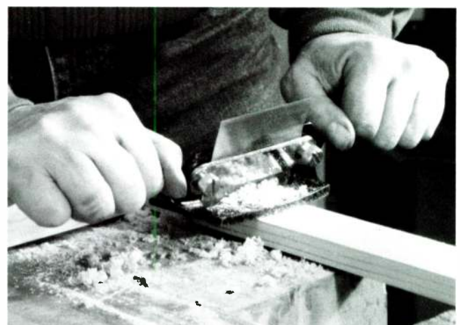
PHOTO 14: Pushing the cabinet scraper to smooth a wood surface.
