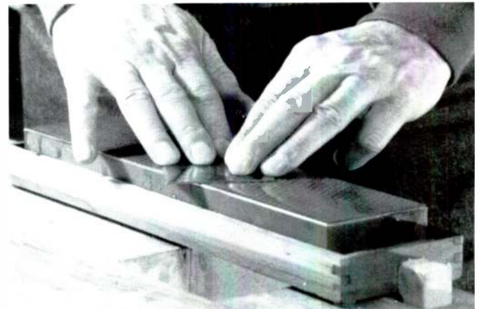
PHOTO 10: Flattening and polishing the blade face of a cabinet scraper.
