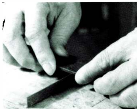
PHOTO 2: Using a mill file to prepare the edge of a hand scraper.
