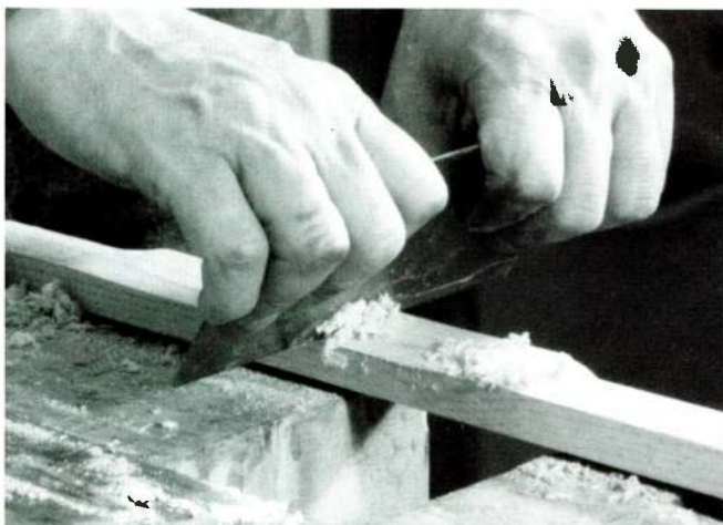
PHOTO 13: Pushing the hand scraper.
