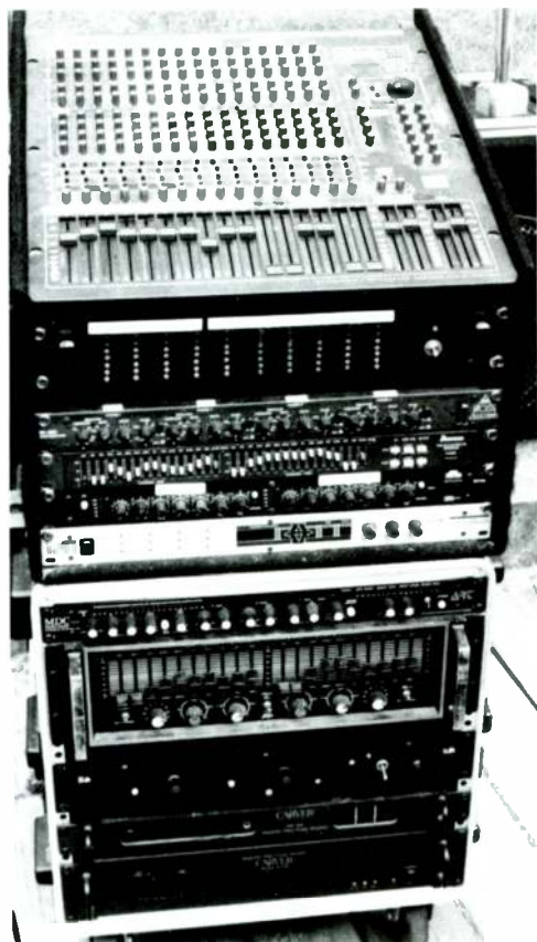
PHOTO 1: Control section for a modern PA system.
