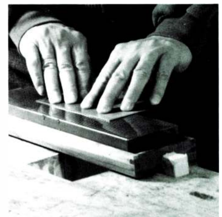
PHOTO 4: Removing the wire edge from a sharpened scraper.
