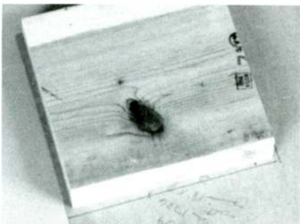
PHOTO 3: Sizing a piece of veneer by placing the surface to be veneered on top. Note that the veneer is cut a little larger than the surface to be veneered.
