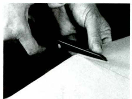
PHOTO 4: Cutting veneer to size using an X-acto knife (upper left), a veneer saw (left), or scissors (right).
