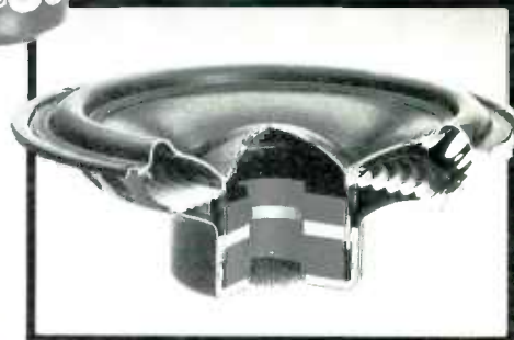
Typical Double Magnet Woofer Cross Section.
