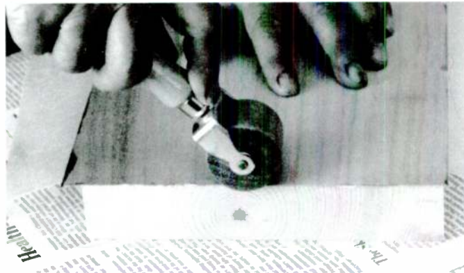
PHOTO 8: Using a small hard roller to anchor the starting seam.
