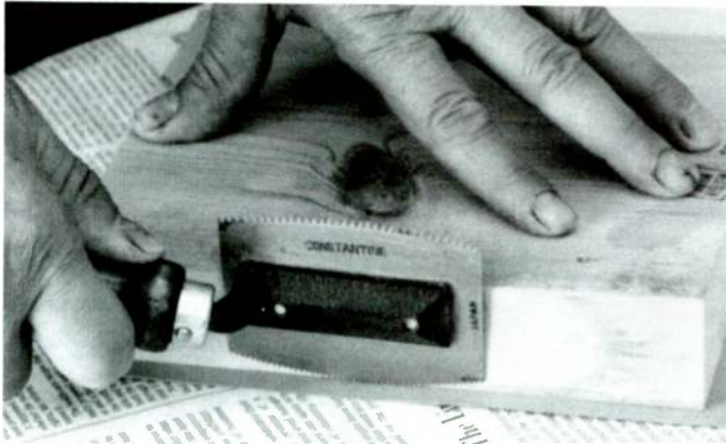
PHOTO 12: Using a veneer saw to remove excess veneer when the veneer grain is parallel to the edge.
