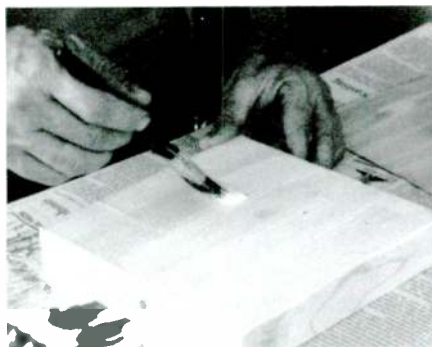
PHOTO 5: Veneer with cement applied and cement being applied to the wood.
