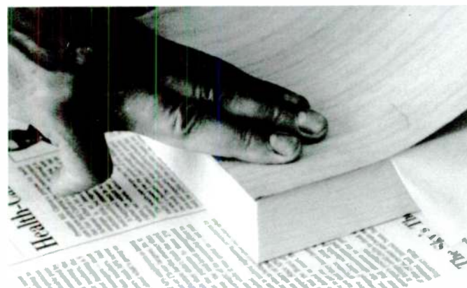
PHOTO 9: Smoothing the veneer after the waxed paper has been pulled out an inch or two.
