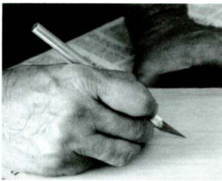
PHOTO 11: Cutting a slit with a sharp knife to repair a blister where the veneer did not stick to the wood.
