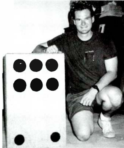
PHOTO 1: The completed cabinet with carpet covering.
