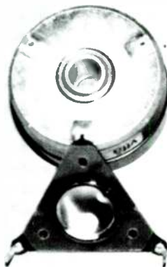
PHOTO 4: D/VC assemblies removed from magnet assembly.
