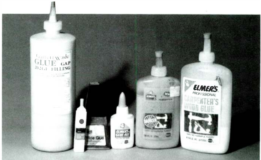
PHOTO 1: Common glues from left to right: Garrett Wade 202GF gap-filling glue (PVA), a superglue, a hide glue (animal glue; poor for speaker enclosures), Elmer's Glue-All (PVA), and two varieties of Elmer's Carpenter's Wood Glue (aliphatic). Another common glue (not shown) is Titebond Wood Glue (aliphatic). The 202GF glue is available from Garrett Wade, 161 Ave. of the Americas, NY, NY 10013-1299, as stock #62J01.03.
