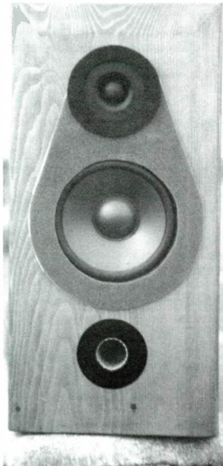
PHOTO 1: Adding foam around the drivers improved these speakers' sound.
