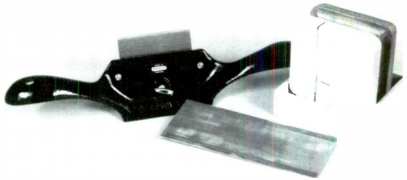
PHOTO 5: Wood scrapers. From left to right: Stanley #80, hand scraper, and a new single-edge razor-blade scraper (Garrett Wade stock #52K08.01).
