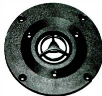
PHOTO 4: D/VC assemblies removed from magnet assembly.
