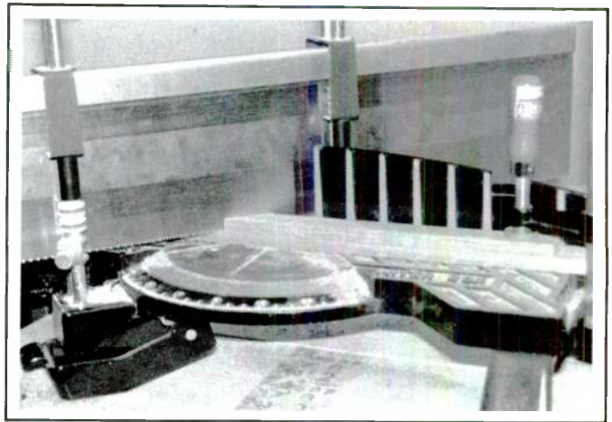
PHOTO 9: Cutting 45° bevels for top trim stock.
