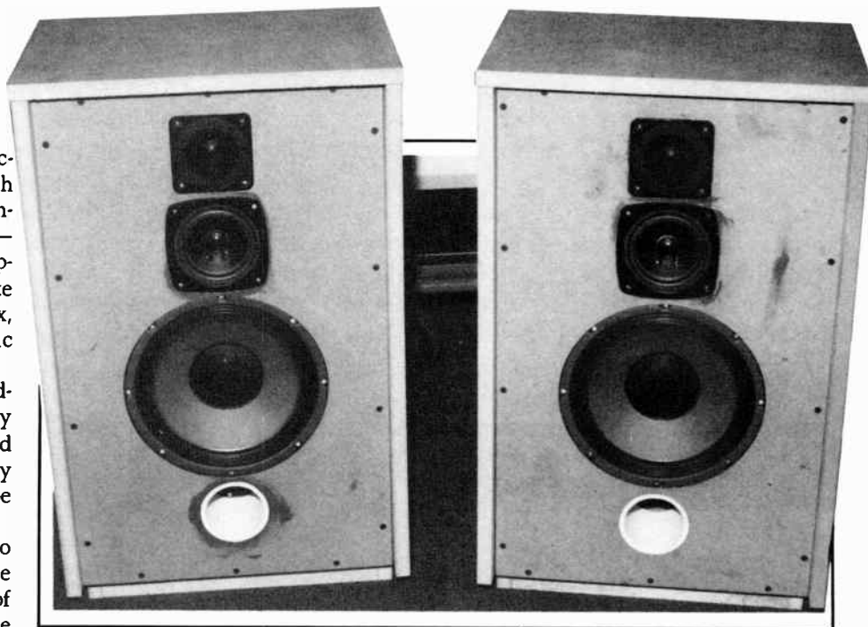
PHOTO 1: These loudspeakers were constructed of fiberboard according to the author's plans, but the front panel is recessed, the top panel is slightly wider, the port is below the woofer and the base is larger. The drivers are those recommended in the parts list.
