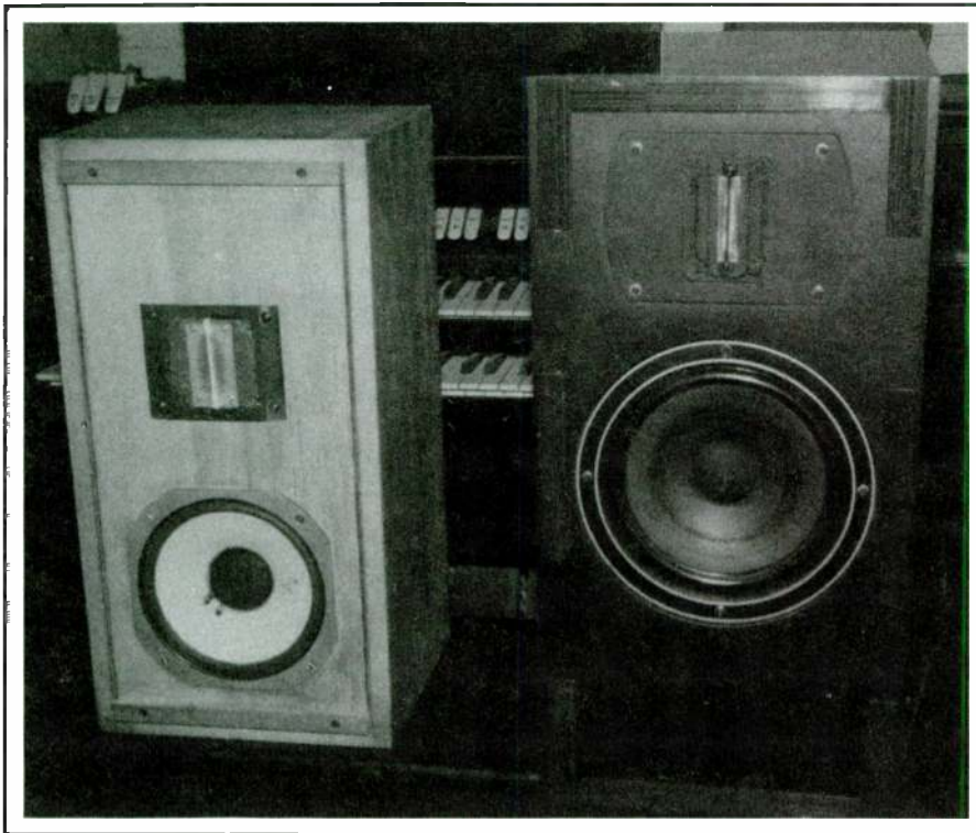
PHOTO 5: Keith Johnson's monitor speakers for his recording sessions. The pine box monitor is on the left, and the "black box" monitor is on the right. Notice the Q-Tip used as a phase divider on the ribbon tweeters. The pipe organ that he is rebuilding is in the background.
