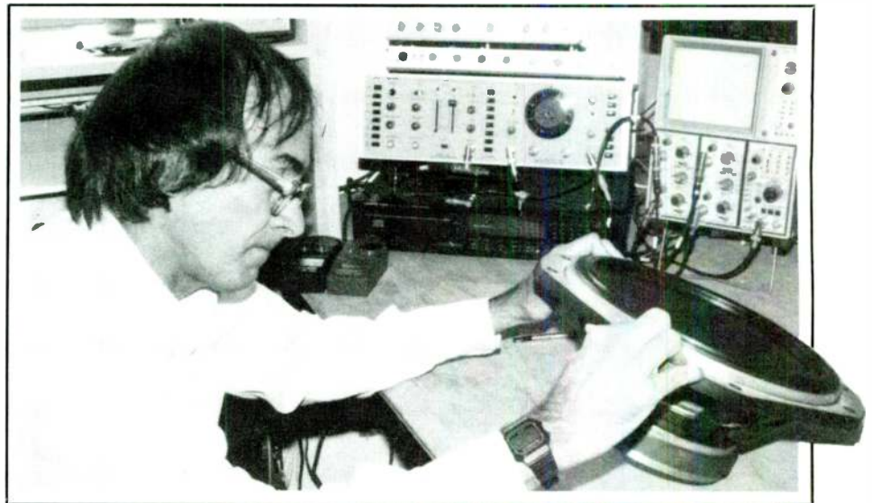
PHOTO 2: Keith examines a driver for excursion and linearity.
