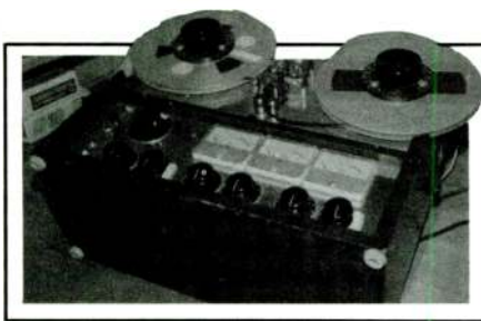
PHOTO 1: The three-track tape recorder used by Keith Johnson in recording sessions for Reference Recordings.
