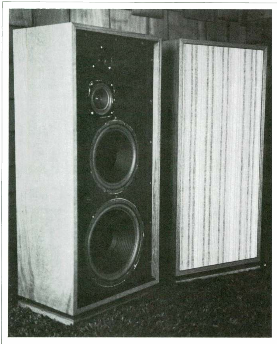
PHOTO 1: The author's three-way system includes a 12" passive radiator.
