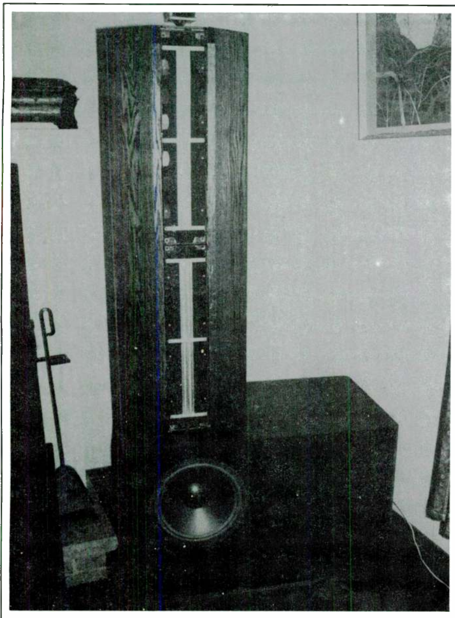
FIGURE 7: A completed JCRC unit with the grilles removed gives you a look at the mounted speakers.
