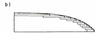
FIGURE 1B: An alternate construction method is to use concentric rings of decreasing radii to form a stepped approximation of the flare. Fill the steps with the "plastic wood" to smooth out the contour.
