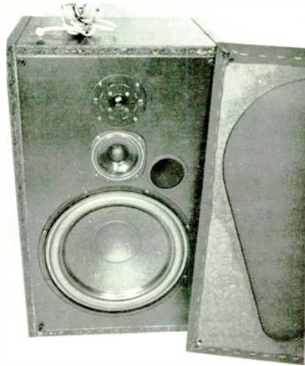
Fig. 8. The completed unit with the grille removed. The 15 ft. cord is #18 stranded type with DIN connector. Grille snaps into place on four posts.
