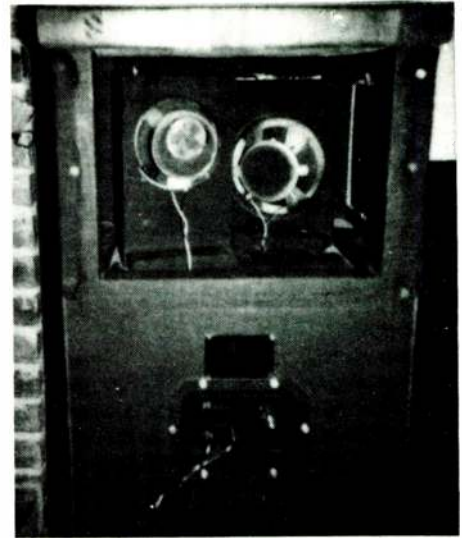
Above, back view of the enclosure showing the two midrange units and terminal board. Below, the laminated top of the cabinet.
