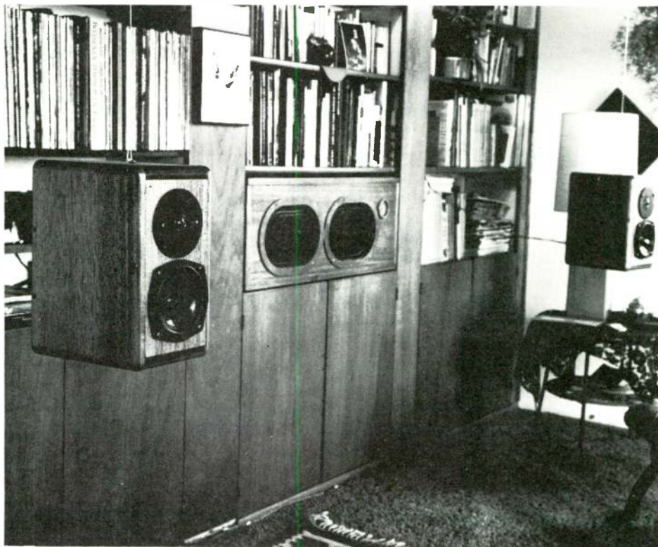
Photo A. Author's system on location. The satellite/midrange tweeter enclosures hang from the ceiling by curtain cord, and remain oriented by the signal cable at the rear of each.
