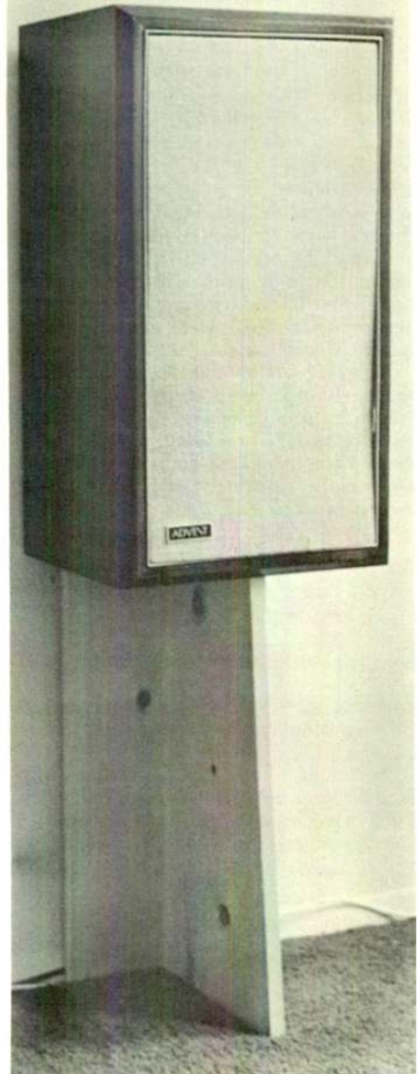
Photo A. Author says rear board should be wider than his prototype—and have tapered shape so the base is two to four inches wider than the top.
