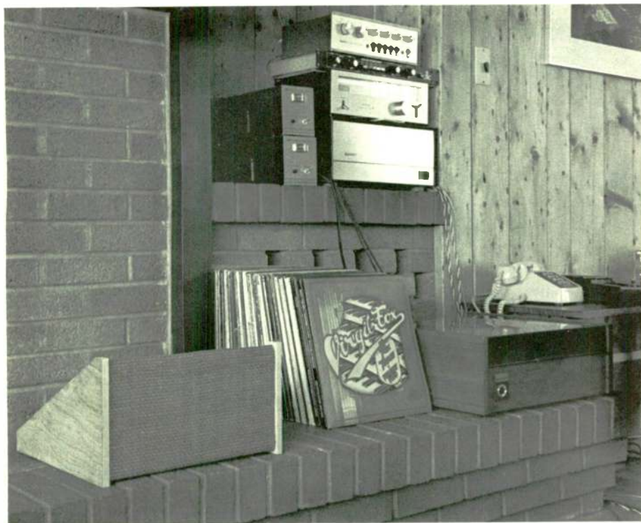
Fig. 2. Preferred orientation: reflecting off wall.
