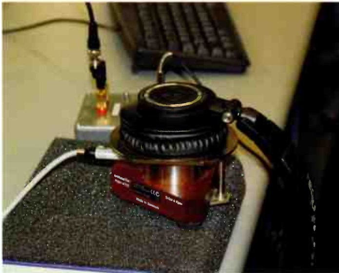
The B&K 'Artificial Ear' test microphone and physical interface with a pair of Audio-Technica MTH-50Ss mounted for evaluation.
