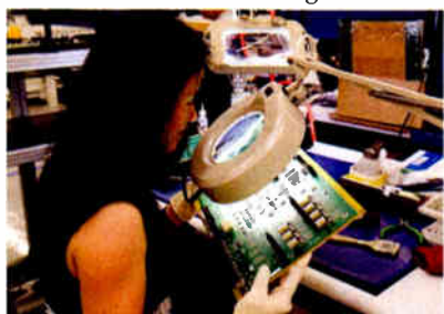
Carefully inspecting PCBs prior to final assembly
