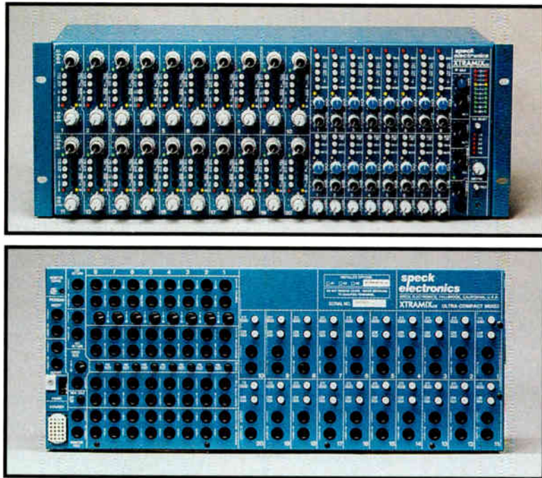
So many inputs so little time: Speck Electronics XTRAMIXcxi synth/line mixer's front (top) and rear offer 76 inputs.
