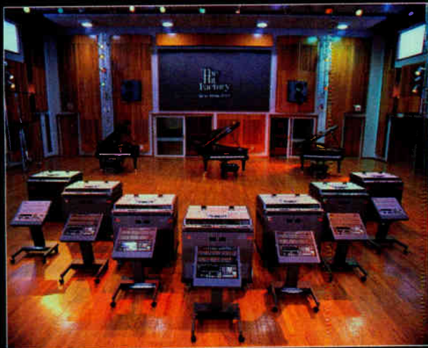
The Hit Factory currently has ten PCM-3348HR machines in its NYC and Miami studios.
