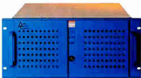
The 55-pound engine boasts dual 500 MHz Pentium III CPUs.
