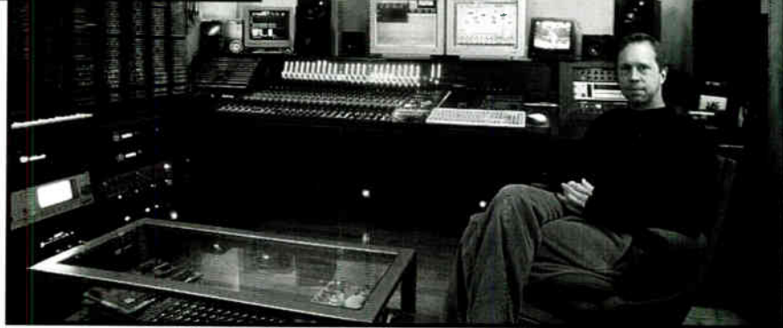
Ed Bair of Bair Tracks, Atlanta, handled the daily voice and music spots for TNT's promo coverage of the NBA playoffs, from his 48-fader Otari Concept I console (with DiskMix moving fader automation) and 32 tracks of Pro Tools. Voice was sent daily from New York via ISDN; the music was an edit of Tears for Fears' "Elemental."
