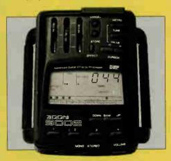
PCM-sampled instruments; transposes; stores songs and patterns (it has a bunch of patterns from the factory to start you off) and remembers what you write.
