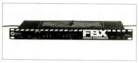
single-channel device, multiple units must be used for stereo mains or to run several different monitor mixes.
