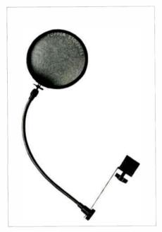
and the clamp holds the gooseneck six inches away from the stand; exact placement can be made with just about any mic/shock-mount combination. Additionally, all of the components use standard 5/8-inch diameter mic stand threading, so the parts could be swapped or rearranged to suit any application.
