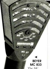
The MC 833 from Bever Dynamic (Hicksville, NY) is a stereo microphone with three cardioid. true-condenser capsules, offering X-Y, unmatrixed M-S and mono outputs. Two outer capsules are adjustable from 60°-180° when used for X-Y recording or summed to a figure-eight output in M-S mode, A front-
