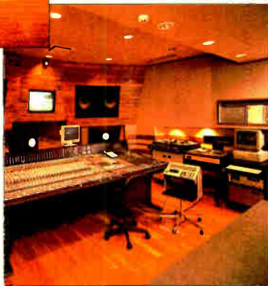
The control room features an automated 36-input DDA DCM232 mixing console, and Sony PCM-3324A and PCM-3402 DASH recorders.
