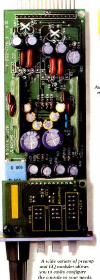
Laser-trimmed resistor packs and 18-turn trim-pots maintain precise circuit tolerances
