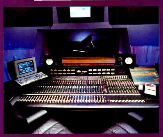
Studio B at Echa Sound of Los Angeles has been fitted with a Trident 80C 32input console with Digital Creations automation Additionally a new Studer A827 24-track tape machine has been added to the room Photo: Kristen Dahline.
