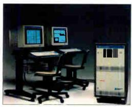
The DSP Option, a 24-bit draital mixer/digital signal processor.
