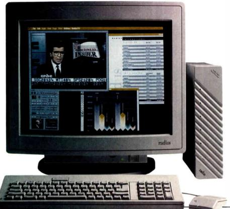
Above: The "pocket accessitor". Paul Brainerd's vision of the computer of the future. Left: Radius TV features a video processing engine, an external audio/video input processor and television tuner that allow display and digitizing of live 16-bit video images at 30 fps on Mac II computers.
