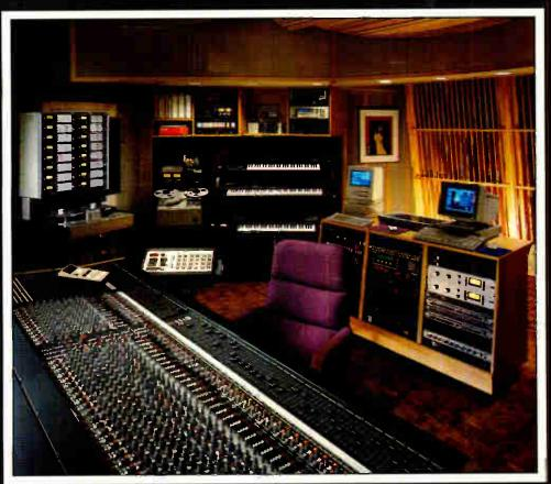
Originally built in 1978 by John Storyk, Horizon Studio was rebuilt late last year by co-owner Vic Steffens with acoustical design assis-tance from Storyk. The centerpiece of the control room is a 44 x 24 Allen & Heath Sigma console with built-in mute automation run trom elther a Mac or an Atari ST. The facility is used for both live and MIDI productions, making use of an adjacent 875 square-foot live room with c 14-foot ceiling and a full MIDI facility in the control room. Photo: Tracey Kroll
