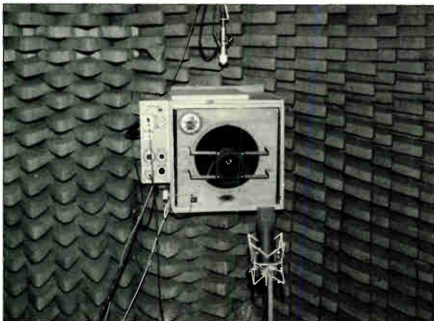
A U69 microphone under test in an anechoic chamber. The test speaker was built by Neumann also.
