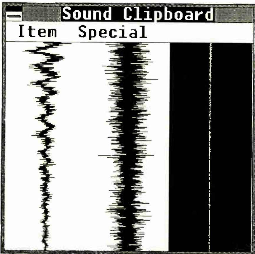
FIGURE 1: AudioFrame's "trim bins" allow sections of audio to be copied, cut, stored, zoomed and rearranged.
