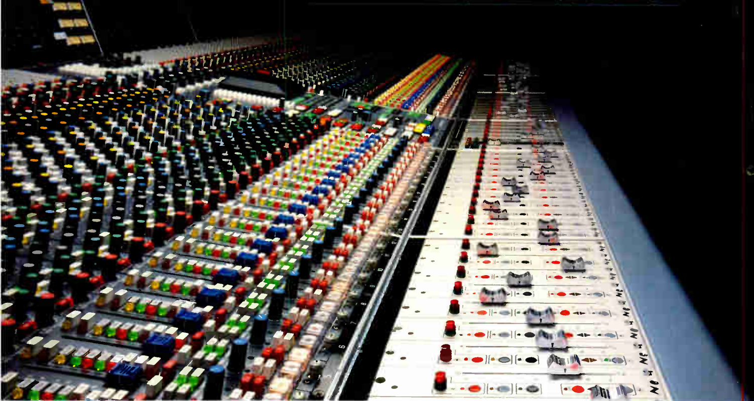
Flying Faders in Neve V Series Console
