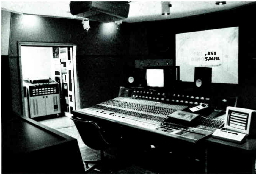
Motown/Hitsville's Dawn Studio is set up to handle audio-for-video mixing and is equipped with an LCRS (left, center, right and surround) monitoring system for Dolby stereo mixdown. Other hardware includes a 40/32 Neve Model 8078 console with Necam 96-fader automation, dual Ampex ATR-124 24-tracks, Ampex ATR-104 4-tracks, Sony PCM-1610 digital processors and an Adams-Smith Model 2600 time code synchronization system with Compact Controllers.
