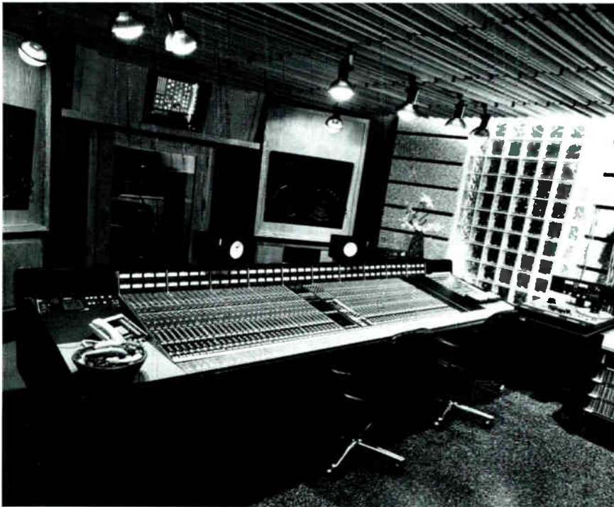
Studio 55's Studio B is equipped with a 72-input Solid State Logic SL4000 E-Series console retrofitted with a G-Series computer and G-Series EQ sections. Like Studio A, the room features Studer A800 multi-tracks and Ampex ATR-102 2-tracks, in addition to a custom TAD monitoring system designed by George Augspurger.
