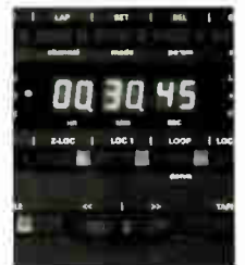
Timer-autolocator control panel
