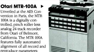
reproduce parameters: level, bias, HF/MF/LF record EQ, phase compensation, HF/LF repro EQ and repro level. Other features include a tilt-down panel with alphanumeric keypad, and backlit LCD display for entering transport and auto-alignment parameters. The VU meter display can be remotely configured, swings up for
