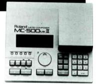
capacity is 100,000 events, with additional storage via the unit's built-in 3.5-inch floppy drive. Another feature is the MC-500 MkII's two independent MIDI outputs for controlling up to 32 MIDI channels simultaneously.
