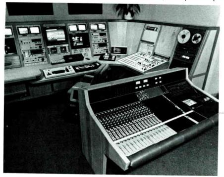
At the Multivision video facility, this custom, automated audio console and the AMS Audiofile are controlled by time code on the master video tape. Digital multi-channel audio—including SFX off CD—mix down directly onto the one-inch master.
