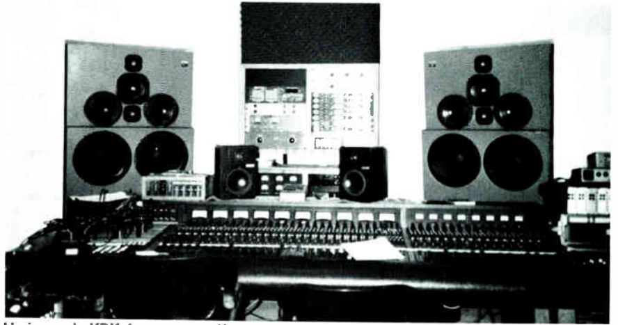
Holman's KRK 4-way monitoring system, custom built by Keith Klawitter.
