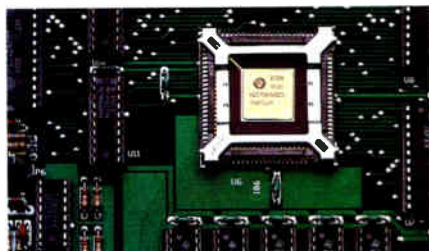
DigiTech's unique custom VLSI chip has 20-bit resolution, and uses innovative HISC processing.
