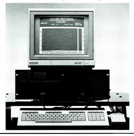
The Kia XZ100's edit screen can display the relative gain levels of up to 32 mixing channels simultaneously. and-white monitor, a 5-pin DIN MIDIspec cable, and a Commodore 5-pin DIN computer-to-monitor cable. A Commodore 128 computer can also be configured to run XZ100 software. The total cost of the C-64 and the C-128 systems is under \$500 and \$800, respectively.
