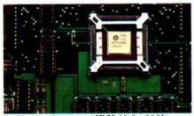
DigiTech's unique custom VLSI chip has 20-bit resolution, and uses innovative HISC processing. The DSP-128 has a master reset function, which restores the
