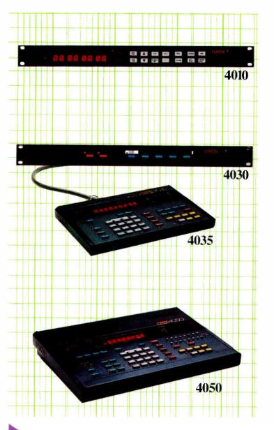
4010 SMPTE Time Code Generator/Reader has all the functions you'll ever need because it's completely software based. As in all high tech digital electronics today, there's a switching power supply. And socketed EPROMs mean your hardware will never be obsolete. Plus, the 4010 has a serial data port on the rear panel which allows communication with (and control by) computers.
