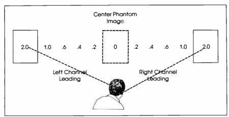
FIG. 2 Approximate image location between loudspeakers versus interchannel time difference in milliseconds.
