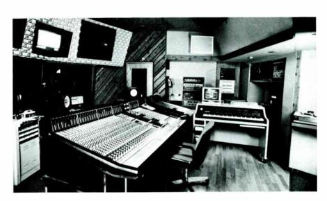
"The Finishing Suite:" SSL with Total Recall mix automation, 5 machine synchronization, 24/48 track to 1" video mixing.
