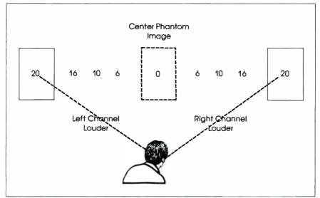
FIG. 1 Approximate image location between loudspeakers versus interchannel intensity difference in dB.
