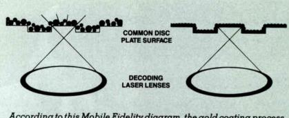
According to this Mobile Fidelity diagram, the gold coating process (shown at right) offers improved reflectivity with fewer "sonic gaps" than standard aluminum coated discs (left).
