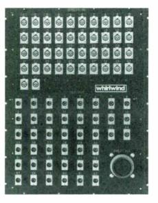
vidually connecting each plug would take quite a bit of time. There are three things to remember when selecting multi-pins. Number one: make sure there are sufficient contacts to accommodate individual ground wires for each channel. Number two: all connector components, (housing, block and contacts), should be made of durable materials. Gold plating on the contacts, while offering a slight conductive advantage initially, is not rec-
