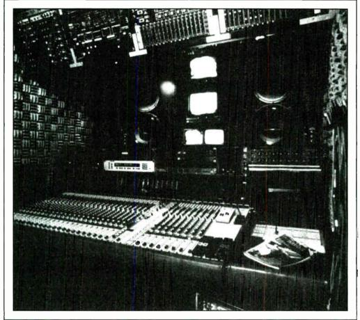
Pictured here: Steven Remote's Aura Sonic Ltd. (ASL) remote truck, based in Flushing, NY, is equipped with a Harrison MR-4 36/32 console, Otari 24-track recorders, a Lynx TimeLine synchronizer, and a full complement of outboard gear, monitor options. microphones and much more. Since 1977, ASL has worked with dozens of audio and video clients on every kind of remote job imaginable. (A story on ASL appears in this issue's remote recording forum, which begins on page 120.) Photo by Steven Remote.
