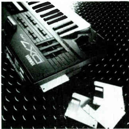
Detail of the DX7IIFD's side-mounted 3.5-inch disk drive.
