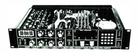
The AMS Model dmx 15-80S was the first digital delay to include sampling capability.
