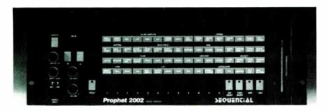
Sequential's Prophet 2002 offers the power of their Prophet 2000 digital sampling keyboard in a MIDI controlled rack mount unit.
