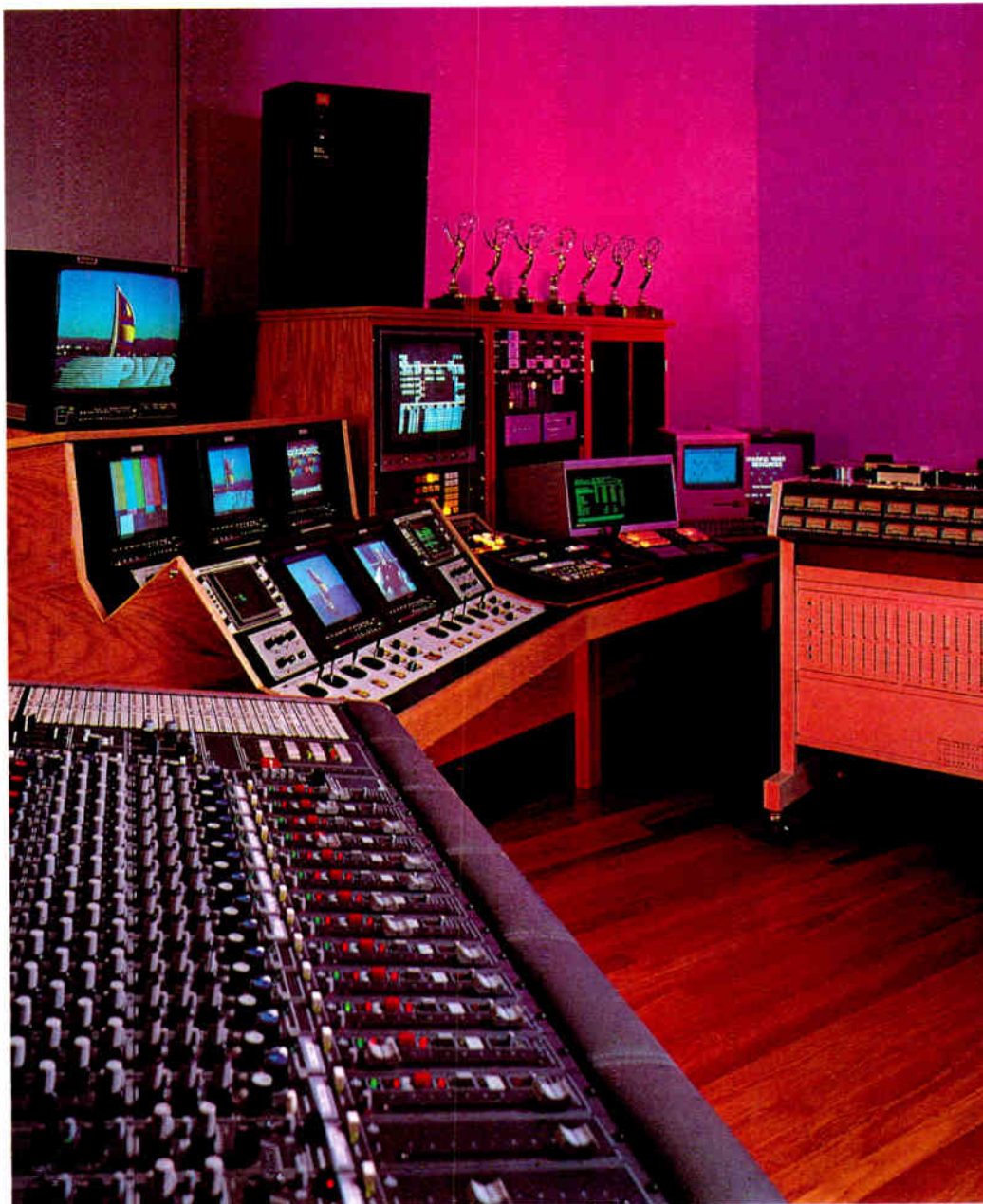
EDIT THREE: 24 channel Sound Workshop 3B mixer with ARMS-II automation; Otari MX 70 16 track audio recorder; Sony PCM 501E5 digital processor; extensive outboard audio processing; Convergence EC S204 computer editor; Sony BVW 15 Dynamic Tracking Betacam players; Sony BVW 40 Betacam recorder; Cox 660 4 band component color correctors; Grass Valley KVC A component video switcher; Intergroup 201 digital matrix wipe generator; Intergroup integrated component composite routing switcher; BVS SA 10, safe title generator.
