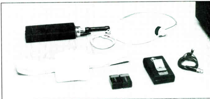
Swintek's Mark QDC/2 system. The QDC receiver (shown here with headset) utilizes the same dB-S companding as the company's top AC-powered units, but its small size makes it ideal for ENG-type on-camera mounting.
