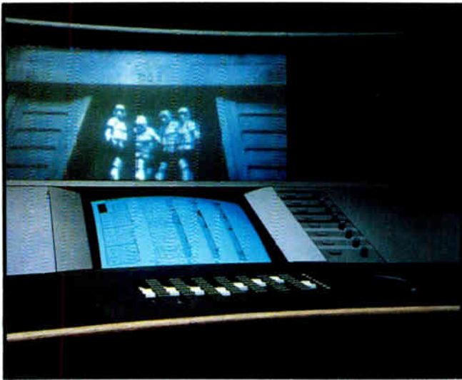
The SoundDroid with visual monitor and "Electronic Cue Sheet."
