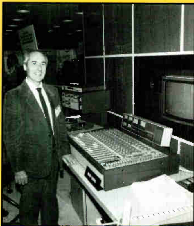
(Below) Senior design engineer John Lumsden with the MXP-2000, Sony's first broadcast console. The board's features include an assignable, four channel dynamics processor; fader start, which can start an ATR when a fader is raised; and an upcoming video editor interface.
