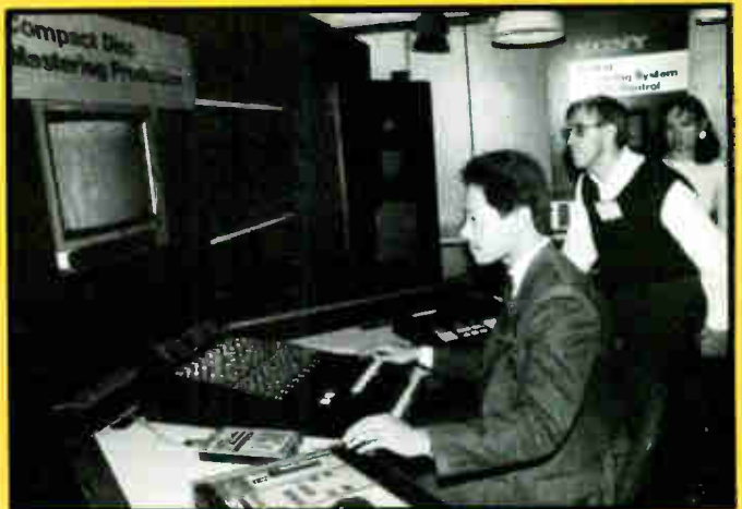
(Below) In the Sony digital suite, Curtis Chan demonstrates CD mastering/prep using the new PCM-1630 processors, DAE-1100 editor and K-1105 digital mixer.
