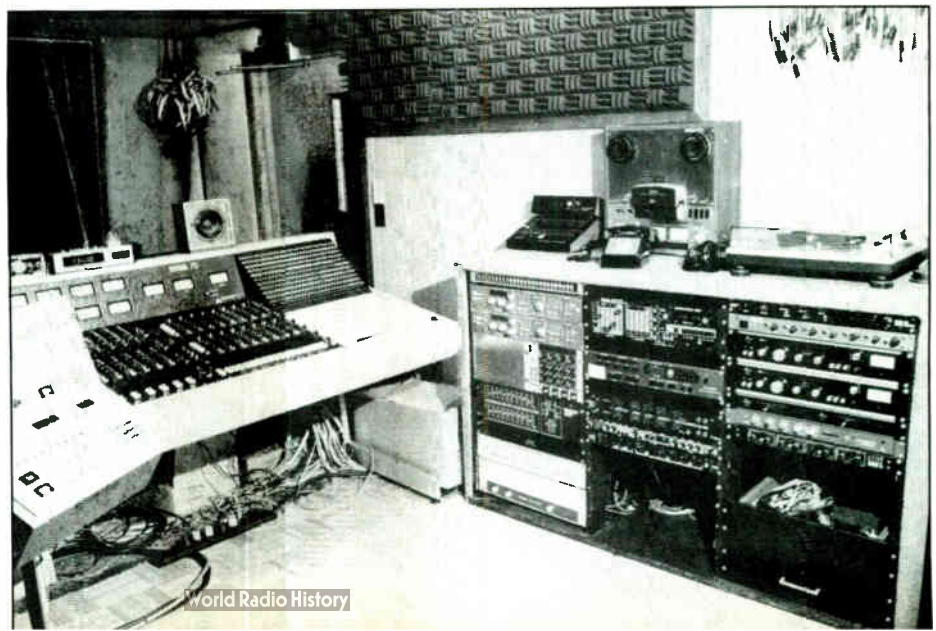
(Left) Showcase Audio/Video Systems' installation at JBS Recording Studio in Atlanta has a number of unique features. The studio is built in an old movie theater, so it has a high ceiling, wood floors and naturally good acoustics. The spacious control room is equipped with an Amek console and two interfaced 16-track Otari MX-70s.
