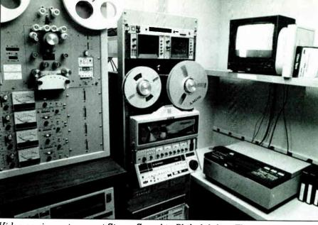
Video equipment room at Sigma Sound in Philadelphia. The studio offers up to 46 tracks of audio and sprocketed mag film transfers to ¾" or one-inch video for sweetening projects.
