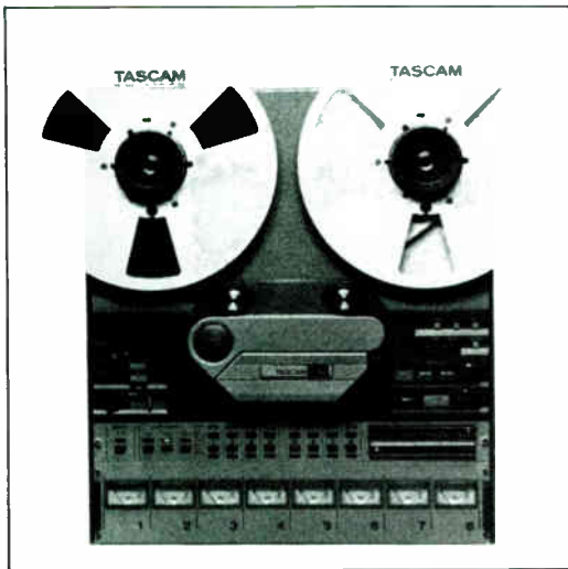
The Tascam Model 58, an 8 track, 1/2-inch recorder, performed well in an audio-for-video environment.
