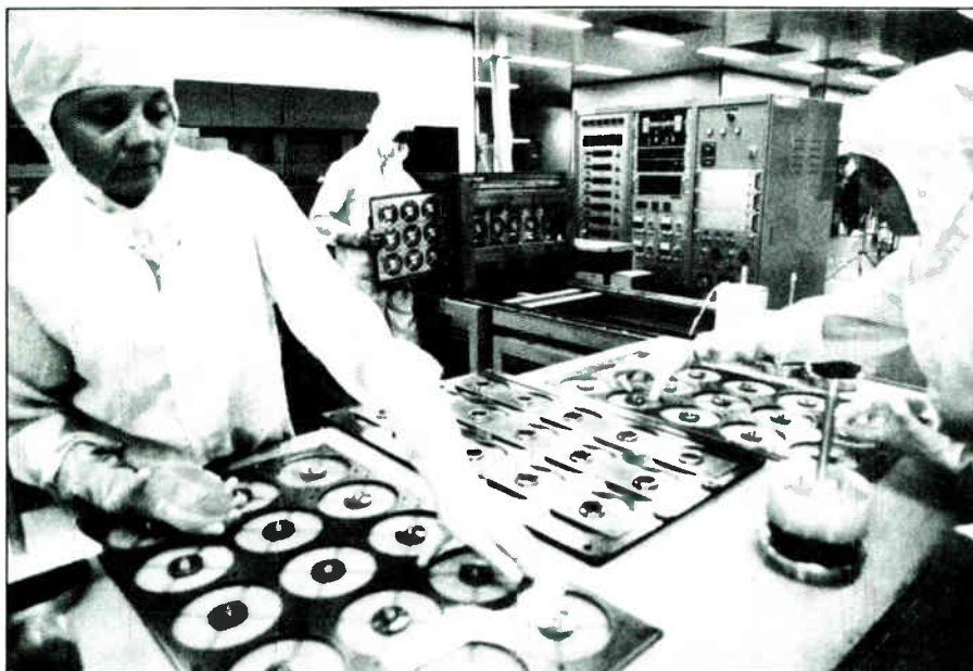
(Above) After injection, a very thin layer of aluminum is placed over the disk's pitted surface that reflects the CD player's laser.
