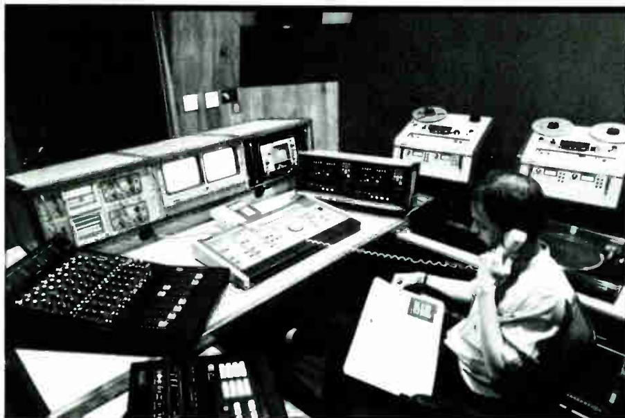
(Left) Compact Disc manufacture starts with a specially encoded tape copy prepared in one of two identical control rooms.
