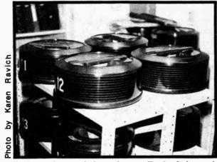
Disk packs used for editing. Each disk pack receives it's information directly from the digital tape recorder. The digital audio information, once on the disk packs, can be edited using the computer.
