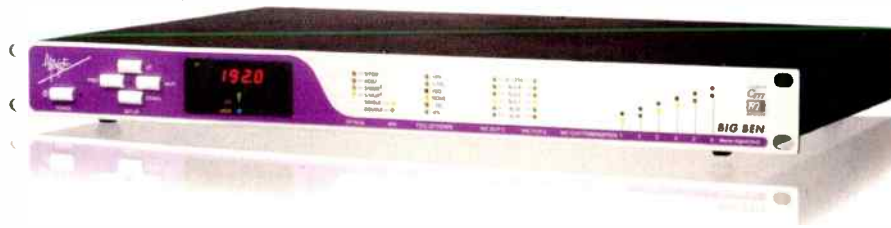
The C777 clock in Apogee's Big Ben Master Digital Clock executes many of the traditional PLL's functions in DSP, attenuating jitter and increasing tolerance of clock-frequency drift.
