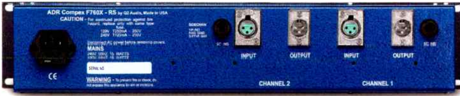
The back panel of the F760X-RS includes XLR in/outs and 1/4-inch sidechain inputs.
