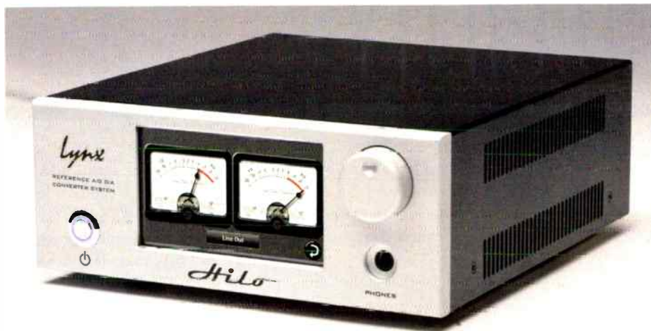
All current Lynx converters use a hybrid PLL circuit called SynchroLock, together with an analog PLL, to reduce jitter in external clock signals. The Lynx Hilo converter is shown here.
