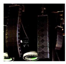
For the main hang, per side, Eighth Day Sound provided ID d&b audiotechnik J8s and four J12s; eight d&b J-Subs; eight d&b V8s for outfill hangs; and, on the ground, six d&b B2 subs per side with eight d&b Qsos for lip fills.
