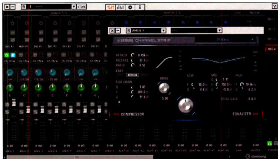
The dspMixFx_UR824 software, showing channel strips and the Sweet Spot Morphing Channel Strip plug-in
