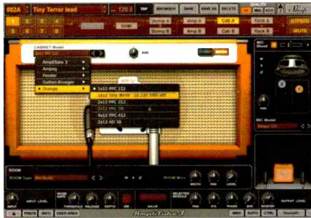
Fig. 2: Pop-up submenus in AmpliTube 3 FREE list models you own, those you're trying and locked models. The remaining trial period for the 1x12 Tiny Terror cab is shown here (highlighted in orange). Two items down in the submenu, the 2x12 PPC OB cab's name is grayed out and has a padlock icon next to it, indicating it is not currently owned or being tried.
