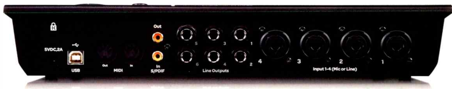
The C600 I/O includes MIDI, USB, S/PDIF line out (six) and mic/line in (four).
