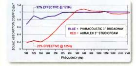
Tests performed by Riverbank Labs on 3" Primacoustic Broadway panels and common acoustic foam. Both absorb high frequencies but as sound shifts to bass, the foam stops working.
