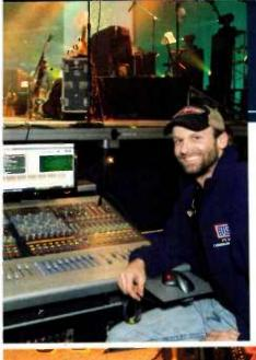
Monitor engineer Jake Bartol is also mixing on a VENUE Profile with a FOH Rack used as a monitor rack and two Stage Racks loaded with 96 analog inputs/16 outputs. Plug ins comprise Fairchild 660 comp on vocals, and D-Verb on vocals and some instruments. "Not a lot," Bartol explains, "I keep it simple."
