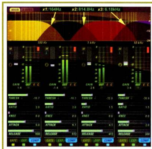
Figure 3: Composite screen from the McDSP ML4000 multiband processor being used to gently limit by about 3 dB (note the red vertical bars). The spectrum has been divided as follows: bass up to 164 Hz, low-mid (164 Hz to 814 Hz), high-mid (814 Hz to 6.18 kHz) and treble (6.18 kHz and above). Threshold, ratio, attack, knee and release can be optimized for each frequency band. EQ can be tweaked via output levels.
