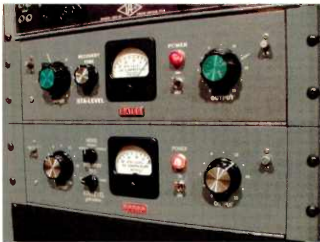
Top: The original Gates Sta-Level unit used on the Johnny Cash record. Bottom: The reissue Retro Sta-Level.
