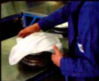
Stretching of the individual glass tissue layers
